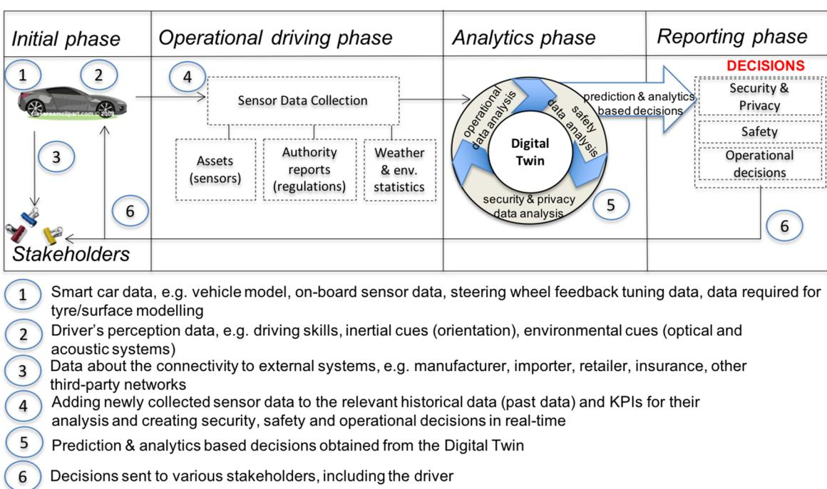
Fig. 1. Smart Car scenario with the Digital Twin.
